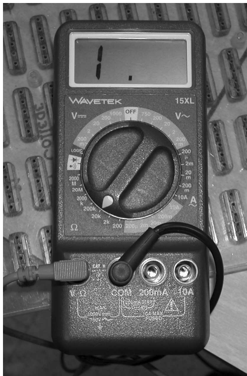
Fig 1: Probe connections for measuring voltage and resistance
