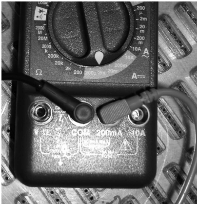
Fig 9: Probe connections for measuring small currents.
