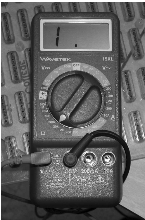
Fig 1: Probe connections for measuring voltage and resistance
