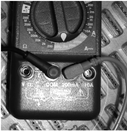
Fig 9: Probe connections for measuring small currents.
