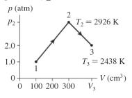
14) The figure shows a *pV* diagram for an ideal gas that is carried around a cyclic process. How much work is done in one cycle if  $p_0 = 4.00$  atm and  $V_0 = 3.00$  L? (1.00 atm = 101 kPa)
