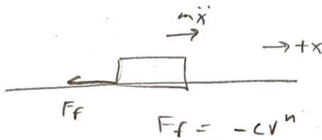
$v = v_0 \text{ at } t=0$  find  $v(t)$ ,  $x(t)$
