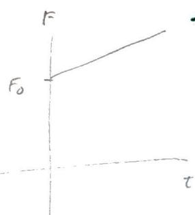
$$\int dv = \int_{0}^t \left( \frac{F_0 + bt}{m} \right) dt = \frac{F_0 t}{m} + \frac{bt^2}{2m}$$
