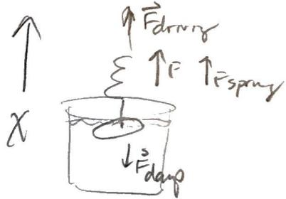
$$\left. \begin{array}{l} \vec{F}_{\text{damp}} = -c\dot{x} \quad \underline{\text{constant}} \\ \vec{F}_{\text{spring}} = -kx \\ F_{\text{driving}} = F_0 \cos \omega t \\ F_{\text{TOTAL}} = m\ddot{x} \end{array} \right\}$$
